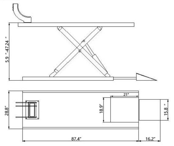
Figure 4 - HYDRAULIC PLAN
