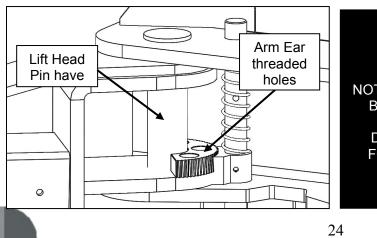
NOTE: EACH ARM RESTRAINT ASSEMBLY MUST BE INSPECTED BEFORE EACH AND EVERY TIME THE LIFT IS OPERATED. DO NOT OPERATE THE LIFT IF ANY OF THE FOUR ARM RESTRAINT SYSTEMS ARE NOT FUNCTIONING PROPERLY.
