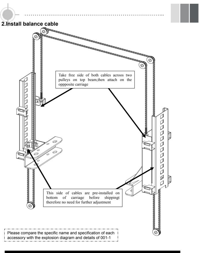
The wire rope should be checked once a week for the same tension, if the tension failure will lead to uneven elevation. The wire rope should be adjusted immediately to maintain equal tension when locked safely.
