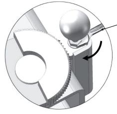
Locking the nuts after the moon gear and arm lock engaged well
