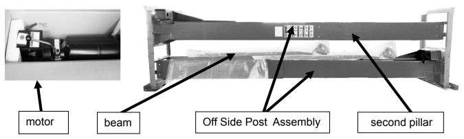
3. Loosen the screws of the upper package stand, take off the upper column and remove the package stand.
