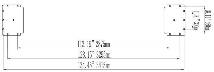
3.Using the base plate on the POWER SIDE post as a guide, drill each anchor hole in the concrete approximately 4.72" deep using a rotary hammer drill and 0.79" concrete drill-bit. To ensure full holding power, do not ream the hole or allow the drill to wobble.
