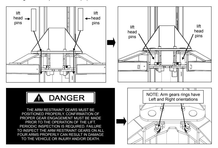
4.Place each Gear Ring against the Lift Head Pin and align the holes in the Gear Ring with the threaded holes in the Arm Ears. Ensure that the teeth on the Gear Ring mesh smoothly with the teeth on the gears of the Lift Head
