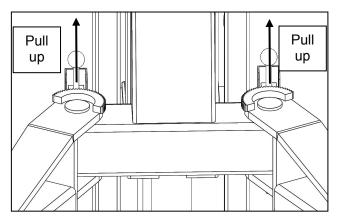
10. Ensure that the arms do not move when a force of approximately 100 pounds or less is applied laterally to the fully extended arms.
