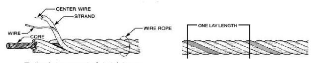
The three basic components of a typical wire rope.
