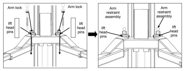
6 pulling up arm lock rod to ensure it is fully unlocked, adjust in this state. Adjust nut as shown
