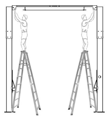
NOTE:Before drilling and anchoring, assemble and install the over head bea
