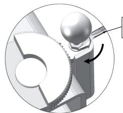
Locking the nuts after the moon gear and arm lock engaged well
