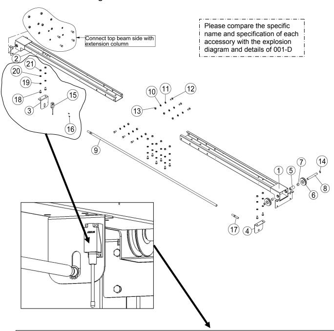
Install limit switch with power unit (Note: The security switch is on the main column side)
